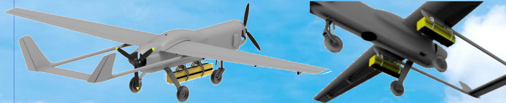
The dropping system can be added under the wings to release a double load or under the fuselage for a single load.
