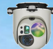
EO/IR cameras can be mounted under the fuselage or under the nose of the drone, as shown above.
